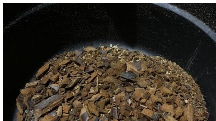
Figure 13. Results of the rough chopping of old coconut fronds at low speed.
