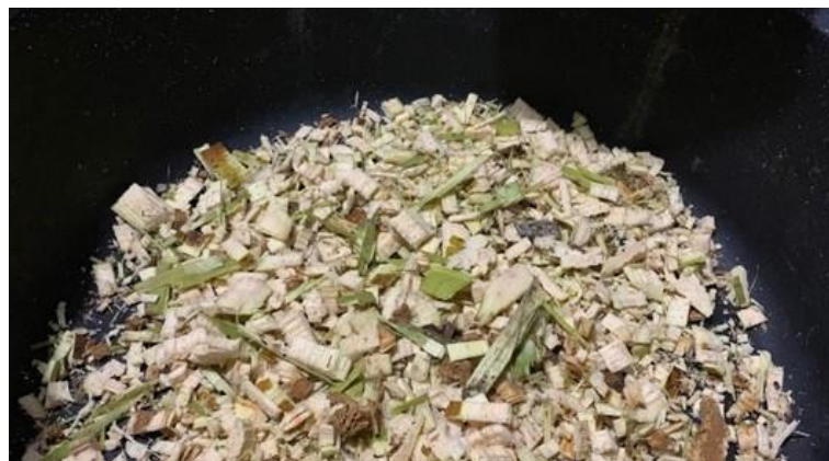
Figure 10. Coarse results of coconut midribs shredding at low speed.
