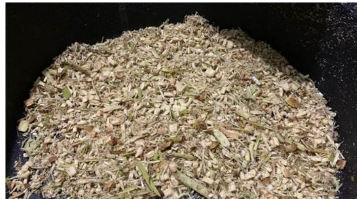
Figure 12. Results of coarse chopping of medium-sized coconut fronds at high speed.
