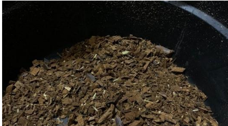
Figure 14. Results of shredding coarse old coconut fronds at medium speed.
