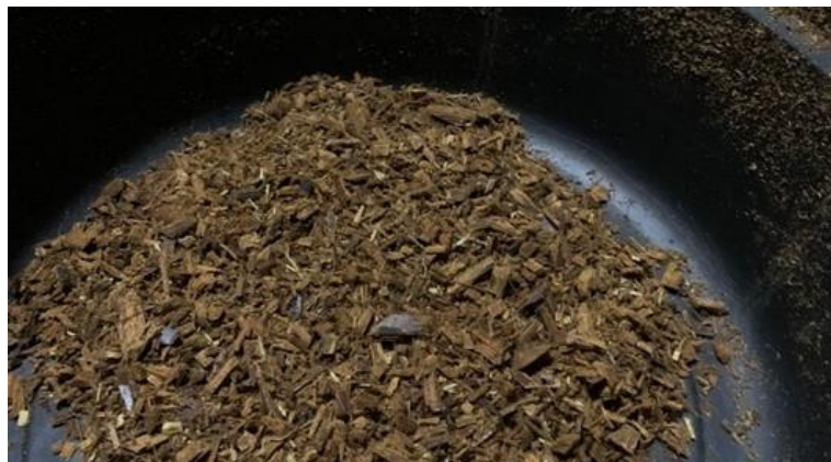
Figure 15. Results of the rough chopping of old coconut fronds at high speed.
