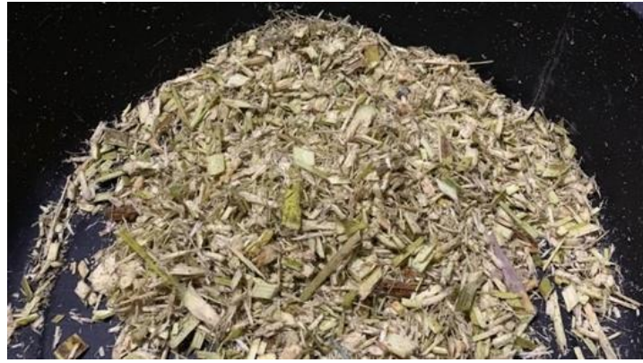
Figure 8. Results of rough chopping of young coconut fronds in the medium setting.
