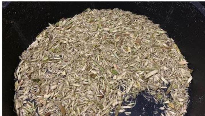
Figure 9. Results of rough chopping of young coconut fronds at high speed.
