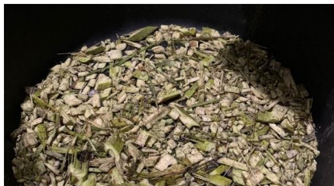
Figure 7. The results of rough chopping of young coconut fronds at low speed.
