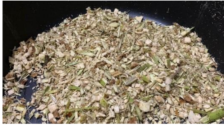
Figure 11. Coarse results of medium-sized coconut frond chipping at medium speed.
