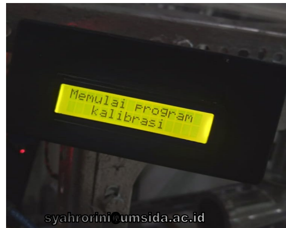
Figure 8. LCD Readout When Load Cell is Calibrated
