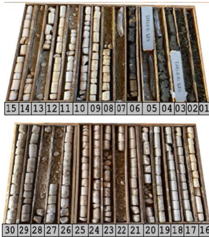
Figure 17. BH1 Borehole log
