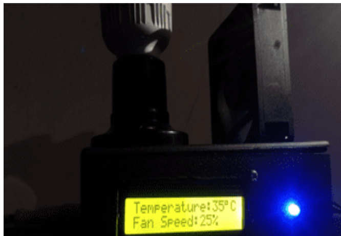
Fig 6. Temperature display 35°C the lights go out and the fans turn on at 25% speed
