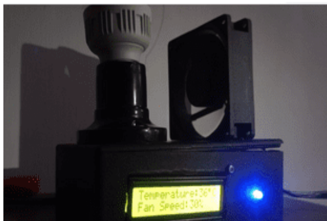
Fig 7. The temperature display is 38°C the light is off and the fan is on at 48% speed
