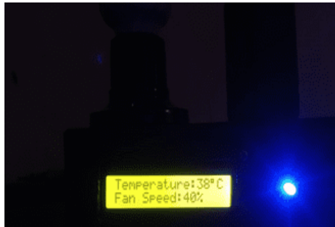
Fig 8. The temperature display is 38°C the light is off and the fan is on at 48% speed
