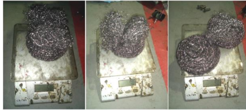
Figure 3. Stainless steel scrap was weighing to 50 g, 70 g and 90 g.
