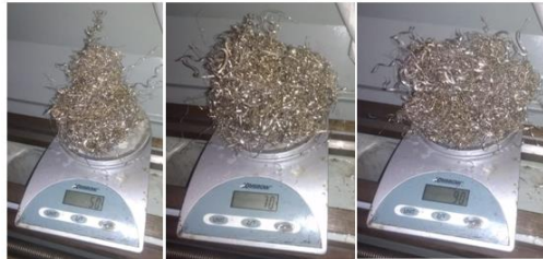
Figure 4. St-40 Iron scrap was weighing to 50 g, 70 g and 90 g
