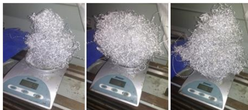
Figure 6. Aluminum scrap was weighing to 50 g, 70 g and 90 g.
