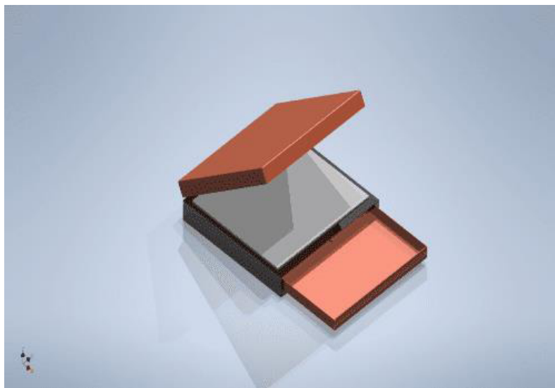
Figure 5 Student engineering results for the mobile case model for the FPGA board
